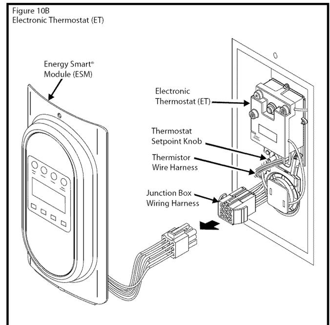
**NOTE:** Smart Grid will be disabled when the Energy Smart® Module (ESM) is disconnected from the junction box wiring harness.
