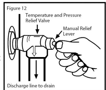
relief valve to allow the valve to operate freely and return to its closed position. If the valve fails to completely reset and continues to release water, immediately disconnect the electrical power, close the cold water inlet valve and call a qualified person.
