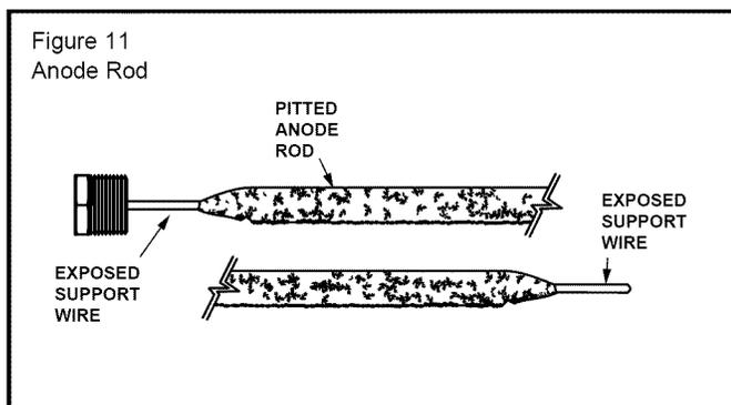
See “Replacing the Anode Rod” in the maintenance section page 15.
