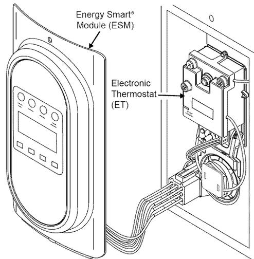
**NOTE:** The Electronic Thermostat (ET) is designed so that it may control the water heater without the Energy Smart® Module (ESM) being operated, see page 12.
