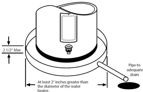
**NOTE:** Local codes and requirements in your area may require the water heater to be installed such that the bottom element is elevated from the floor at least 18 inches.
