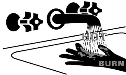
**Water temperature over 125°F can cause severe burns instantly or death from scalds.**
