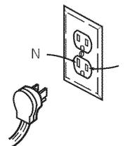
Ensure proper ground and firm connection before use
