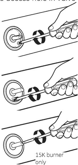
**D** Make the adjustment by slowly turning the screw until flame appearance is correct.
