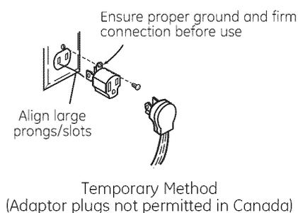
**▲ CAUTION:** Attaching the adaptor ground terminal to the wall receptacle cover screw does not ground the appliance unless the screw is metal, and not insulated, and the wall receptacle is grounded through the house wiring. The customer should have the circuit checked by a qualified electrician to make sure the receptacle is properly grounded.
