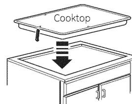
bracket into the cabinet sides to secure the unit into place.
