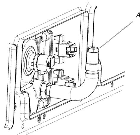
8. Position the back of the bake burner over the oven orifice, and slide the tab on front of the bake burner into the front of the oven.
