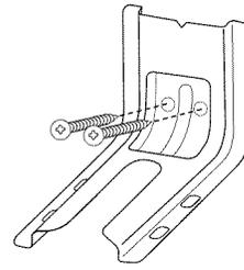
5. Using the Phillips screwdriver, mount anti-tip bracket to the wall or floor with the two #12 x  $1\frac{1}{8}$ " screws provided.
