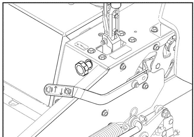
Release the parking brake to restart movement
