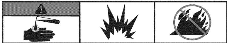
Battery acid is corrosive, explosive and flammable
