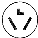
3-wire receptacle (10-30R)
