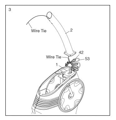
Tip: Avoid pinching the wires. Set the Upright (2) on the Frame (1).
