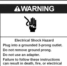
shock. If codes permit and a separate ground wire is used, it is recommended that a qualified electrician determine that the ground path is adequate.
