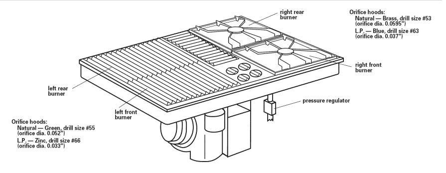
Gas conversions (from Natural gas to L.P. gas; or from L.P. gas to Natural gas) must be done by a qualified installer.
