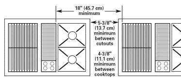
Minimum spacing shown is required for satisfactory performance when installing the
