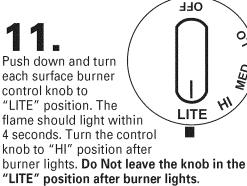
Check each surface burner for proper flame at "HI" setting. The small inner cone should have a very distinct, blue flame that is 1/4" (0.6 cm) to 1/2" long (1.3 cm). The outer cone is not as distinct as the inner cone. Turn surface burner control knobs to "OFF" position.
