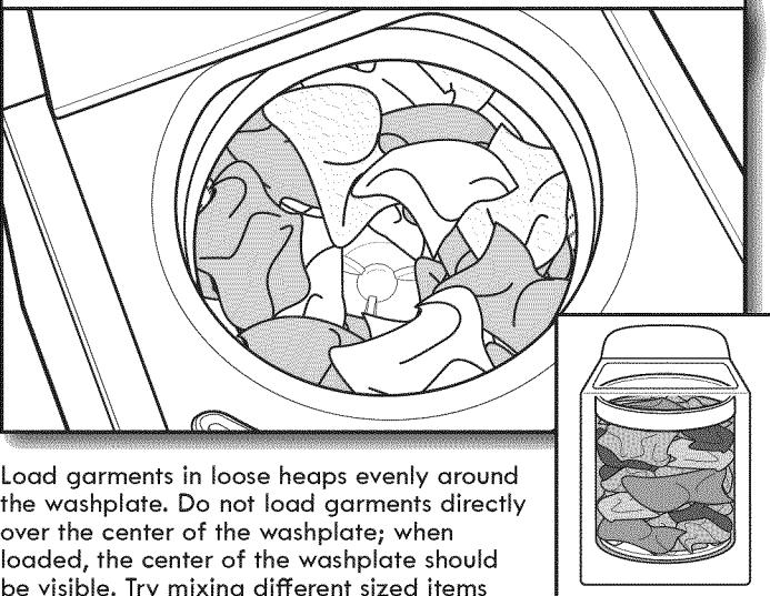
Load garments in loose heaps evenly around the washplate. Do not load garments directly over the center of the washplate; when loaded, the center of the washplate should be visible. Try mixing different sized items to reduce tangling.
