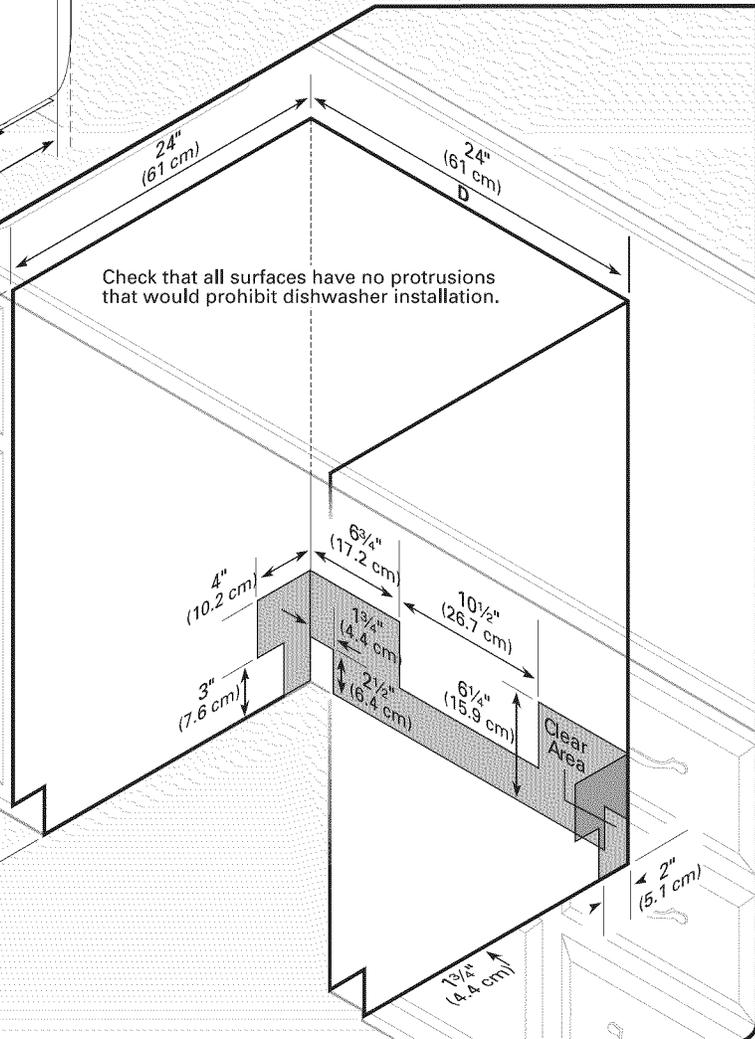
Check that all surfaces have no protrusions that would prohibit dishwasher installation.
