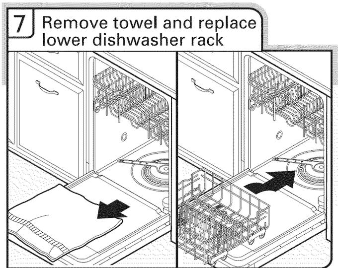
Remove towel from dishwasher. Reinstall the lower dish rack. If needed, see website for animated representation of this step. Visit [www.jenn-air.com/anchoring](http://www.jenn-air.com/anchoring) under FAQ tab.
