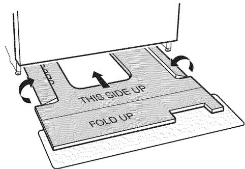
4. Fold the front end of the pad up into position. Make sure the vinyl pad is tucked up behind the door and the dishwasher front legs, as shown.
