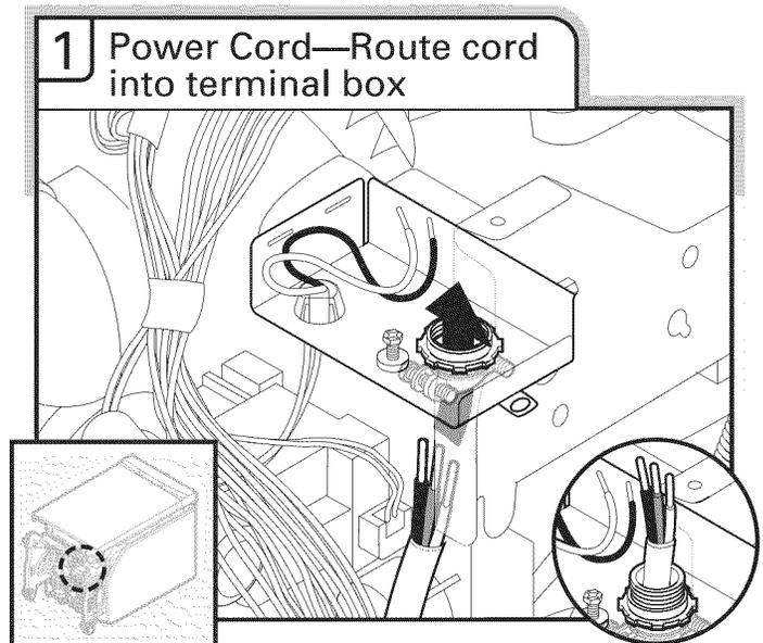
Route cord so that it does not touch dishwasher motor to lower part of dishwasher tub. Pull cord through strain relief in terminal box.
