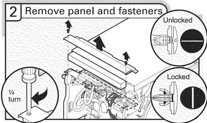
Using a flat-blade screwdriver, turn the plastic fasteners  $\frac{1}{4}$  turn to unlock them. Remove panel. Do not remove tech sheet from access panel.
