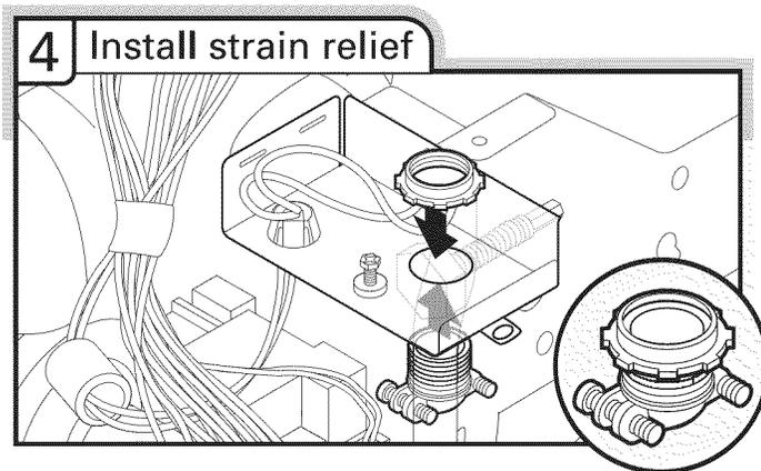
Install a UL Listed/CSA Approved strain relief. Make sure screw heads are facing to the left when tightening conduit nut. Strain relief is provided with the power supply cord kit.
