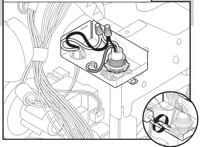
Tighten strain relief screws to secure cord.
