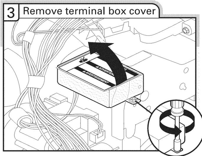
Using a  $\frac{1}{4}$ " hex head socket, nut driver or Torx® T20® screwdriver, remove terminal box cover. Retain for later use.
