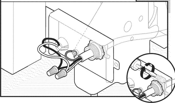
Tighten strain relief screws to secure cable.
