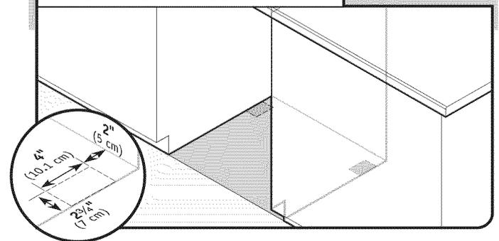
**Built-up floors:** If the kitchen floor is higher than the cabinet opening's floor - for example, the kitchen floor tile does not extend into the cabinet opening - add shims as needed in the area shown to bring the dishwasher up to 34" (86.4 cm) below the countertop.
