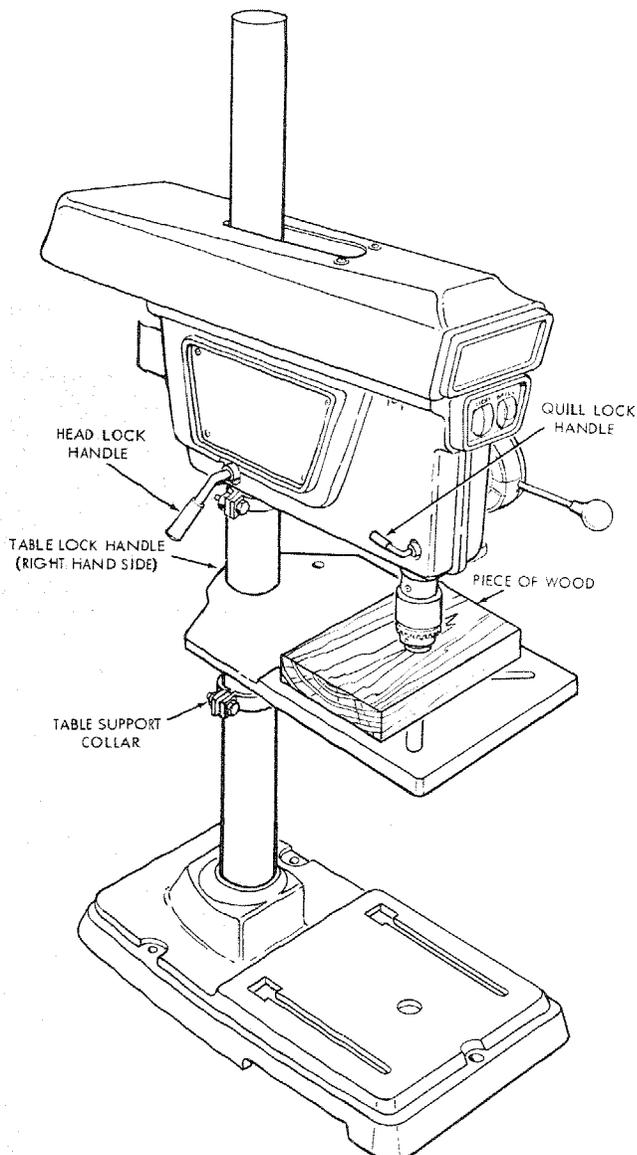
9. Gently push down on the FEED HANDLES until the head raises upwards as far as it will go.
