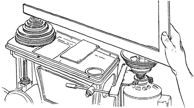
3. Place the belt on the pulleys.
