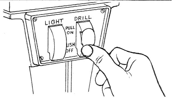
TO lock switch in OFF position ... hold switch IN with one hand ... REMOVE key with other hand.
