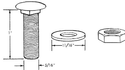
3. Insert the bolts as shown . . . install washers . . . screw on nuts but DON'T TIGHTEN them.
