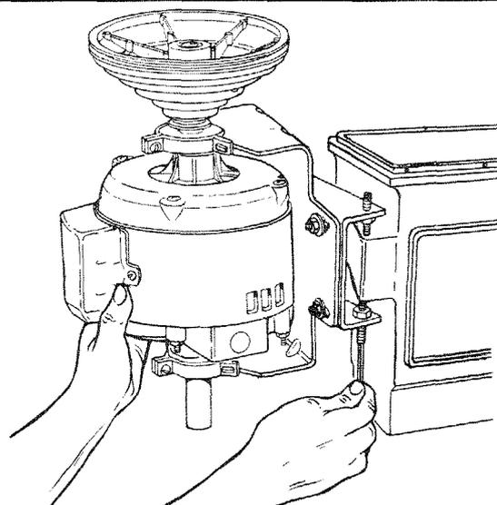
7. Find two 5/16 in-18 hex. nuts among the loose parts ... screw them on to the pivot screws ... tighten them with a 1/2 in. wrench while preventing the pivot screws from turning.
