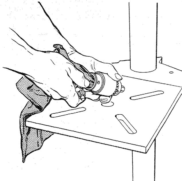
2. Apply a light film of oil such as Sears household oil to the spindle nose.
