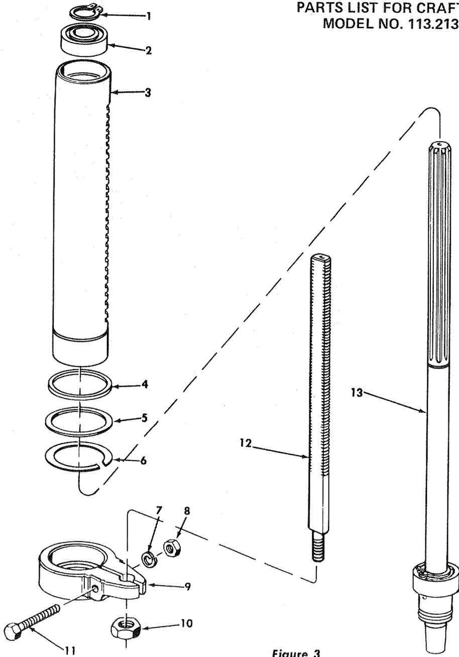
FIGURE 3 – 71075 SPINDLE ASSEMBLY, STOP
