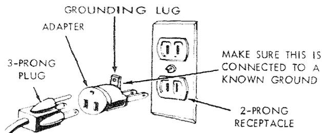
**NOTE:** The adapter illustrated is for use only if you already have a properly grounded 2-prong receptacle. Adapter is not allowed in Canada by the Canadian Electrical Code.
