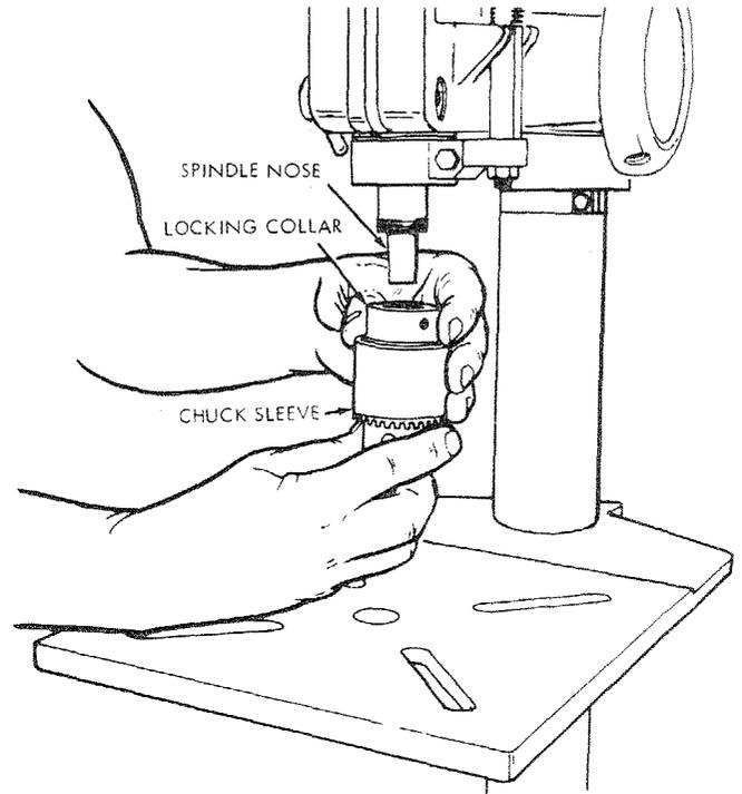
4. Insert a piece of 1/4" dia. STEEL ROD in to one of the holes in the chuck body.
