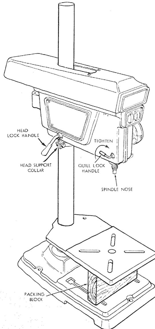
IN ORDER TO RAISE THE HEAD TO A HIGHER POSITION, IT WILL BE NECESSARY TO INSTALL SEVERAL PARTS.
