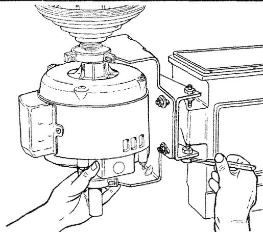
9. Find the plastic CORD TIE among the loose parts ... insert the pointed end into the hole in the motor mount.
