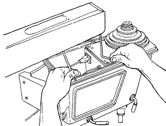
6. Place motor on drill press ... screw the pivot screws into the holes.
