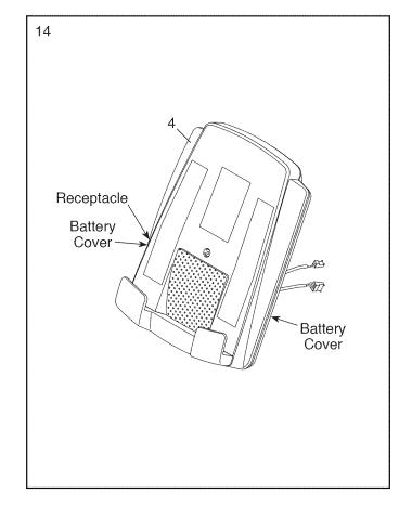
15. While a second person holds the Console (4) near the Console Plate (11), connect the wires on the Console to the Main Wire (53) and to the Pulse Wire (22).
