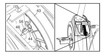
Next, rotate the Pulley (43) until a Magnet (44) is aligned with the Reed Switch (46). Slide the Reed Switch slightly toward or away from the Magnet. Then, retighten the M4 x 16mm Screw (56).
