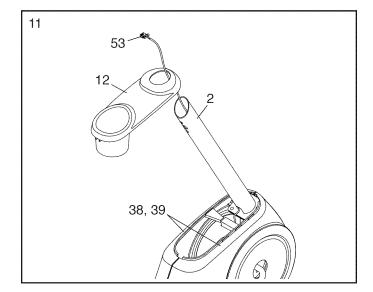
12. Orient the Console Plate (11) as shown. Then, insert the Main Wire (53) upward through the Console Plate.
