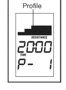
When you select a preset workout, a profile of the resistance levels of the workout will scroll across
