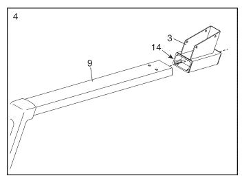
5. Tighten the Adjustment Knob (14) on the Seat Carriage (3).
