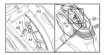
Next, rotate the Pulley (43) until a Magnet (44) is aligned with the Reed Switch (46). Slide the Reed Switch slightly toward or away from the Magnet. Then, retighten the M4 x 16mm Screw (61).
