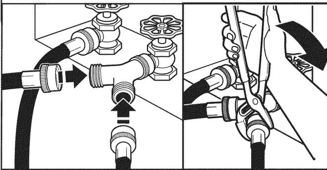
One end of the long hose has a wire mesh strainer inside the coupling. Attach this end to the "Y" connector. Attach washer cold inlet hose to other side of "Y" connector. Screw on coupling by hand until it is seated on connector. Using pliers, tighten the couplings an additional two-thirds turn.
