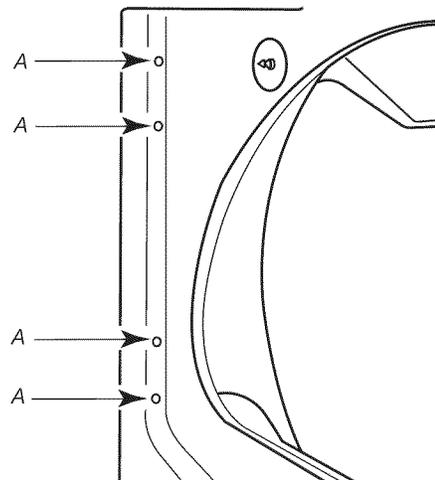
6. Install 4 plastic plugs (A) into screw holes in the dryer left where the hinges were removed in Step 4.
