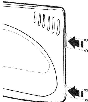
4. Install the two hinges to the front panel of the dryer using 4 screws. Use the non-slotted side to attach the hinge to the front panel.
