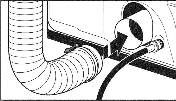
Using a 4" (102 mm) clamp, connect vent to exhaust outlet in dryer. If connecting to existing vent, make sure vent is clean. Dryer vent must fit over dryer exhaust outlet and inside exhaust hood. Check that vent is secured to exhaust hood with a 4" (102 mm) clamp.
