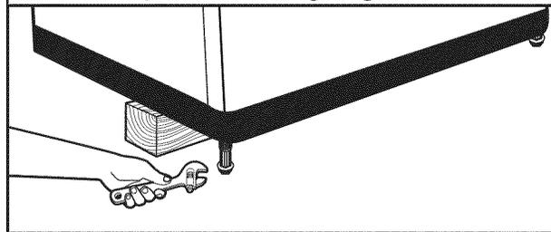
If dryer is not level, prop up using a wood block, use wrench to adjust legs by backing out the foot as needed, then checking again for levelness. Once legs are level, make sure all four legs are snug against the floor.
