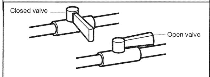
Open shut-off valve in supply line; valve is open when handle is parallel to gas pipe. Then, test all connections by brushing on an approved noncorrosive leak-detection solution. Bubbles will show a leak. Correct any leaks found.
