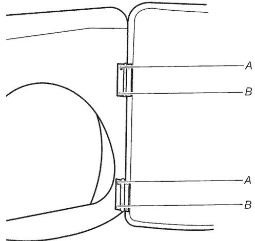
4. Remove the dryer door and the hinges by lifting upward on the door. Lay the door on a flat, covered surface, with the inside of the door facing up. Remove remaining two loose screws from dryer front panel.
