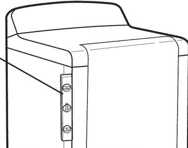
Check levelness of dryer from side to side. Repeat from front to back.
