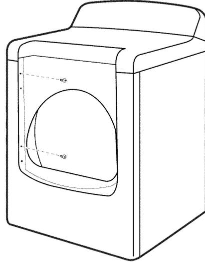
6. Hang door by placing screw heads into top slotted holes of hinges and slide door down. Align bottom screw holes in hinge and door. Install two bottom screws. Tighten all hinge screws.
