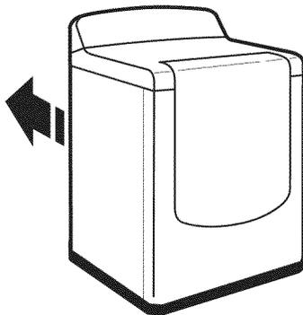
Move dryer to final location. Avoid crushing or kinking vent. After dryer is in place, remove cardboard from under dryer.
