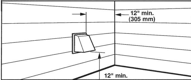
Install exhaust hood and use caulking compound to seal exterior wall opening around exhaust hood.
