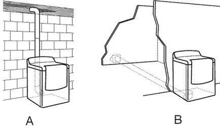
A. Standard rear offset exhaust installation
