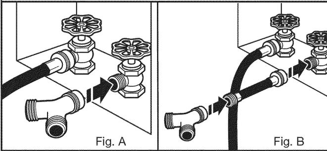
If space permits, attach the female end of the "Y" connector to the cold water faucet. See figure A.
