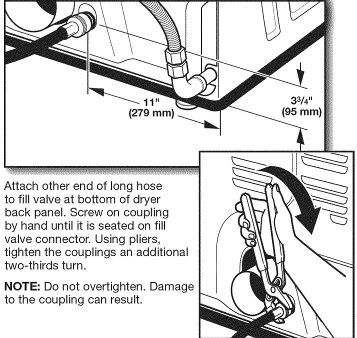
Attach other end of long hose to fill valve at bottom of dryer back panel. Screw on coupling by hand until it is seated on fill valve connector. Using pliers, tighten the couplings an additional two-thirds turn.
