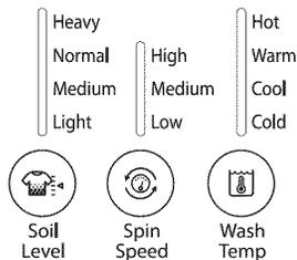
Once you select a cycle, the default settings for that cycle will be lit. Press the cycle modifiers buttons to change the Soil Level, Spin Speed, and Wash Temp, if desired. Not all settings are available with all cycles.
