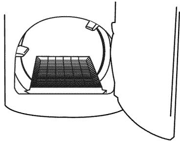
2. Align the two hooks on the front of the drying rack with the holes in the dryer door opening and press down fully into holes. Rest the rear support on the dryer back ledge.
