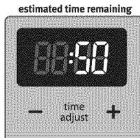
When you select a Timed Cycle, the default time appears in the display. Use the + and - buttons to increase or decrease the time in 1 minute increments. Press and hold to change the time in 5 minute increments. The maximum dry time is 100 minutes.
