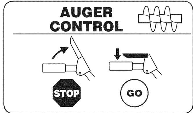
The auger control is located on the left handle. Squeeze the control grip against the handle to engage the augers and start snow throwing action. Release to stop.
