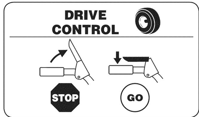
The drive control is located on the right handle. Squeeze the control grip against the handle to engage the wheel drive. Release to stop.
