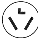
3-wire receptacle (10-30R)
