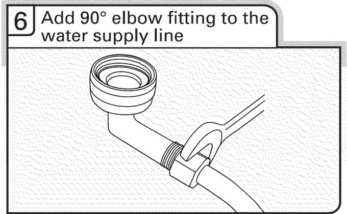
Connect the  $\frac{3}{8}$ " compression fitting to the water supply line prior to installing the unit into the cabinet opening. Attach such that the  $\frac{3}{4}$ " connection is facing upward as shown above.
