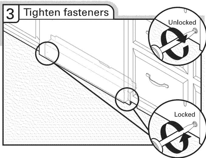
Using a flat-blade screwdriver, turn the fasteners  $\frac{1}{4}$  turn to lock into place. The fasteners slot will be straight up and down when properly locked.
