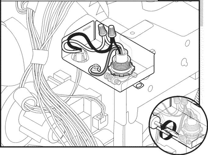
Tighten strain relief screws to secure cord.
