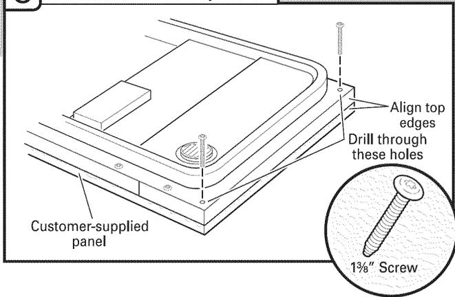
Install the two #8-18 x 1 1/8" screws from the literature package in the top corners of the inner panel. Tighten the six side screws reinstalled in Step 6.
