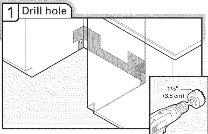
If needed, drill a  $1\frac{1}{2}$ " (3.8 cm) diameter hole in cabinet wall or side of the opening closest to the sink.
