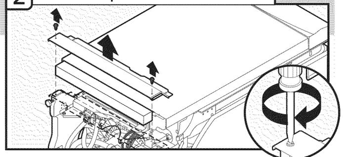
Using a flat-blade screwdriver, turn the plastic fasteners ¼ turn to unlock them. Remove panel. Do not remove tech sheet from access panel.
