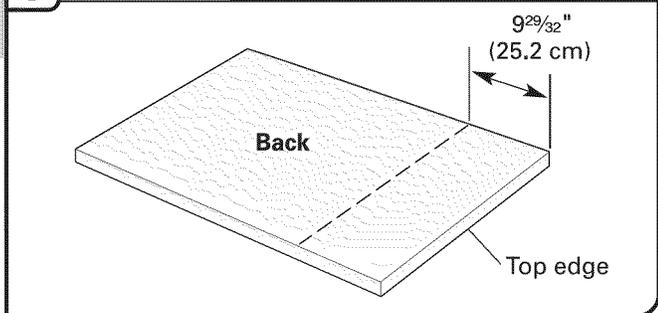
Measure 9<sup>29</sup>/<sub>32</sub>" (25.2 cm) from top edge and mark a line on the back of customer-supplied custom panel. Position the outer panel on the back of the customer-supplied custom panel as shown, so that the top holes in the outer panel are on the line, and both panels are centered side to side.
