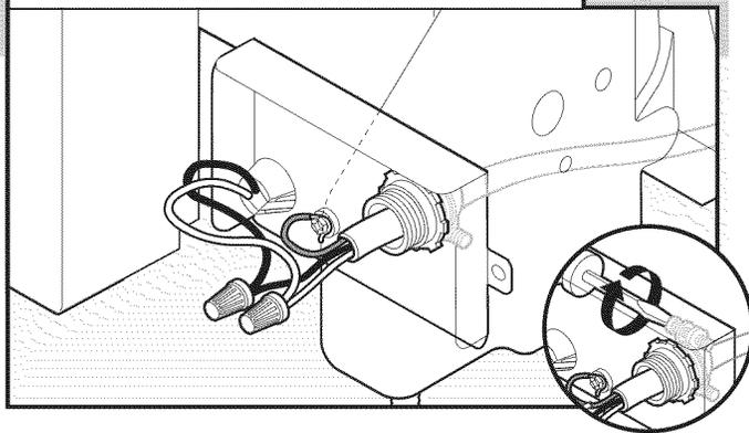
Tighten strain relief screws to secure cable.
