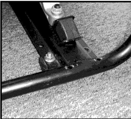
This generator has an option of not using the mobility kit. If this is desired, just install the 4 rubber mounts on the frame as shown. (this is why there are 6 mounts). If you want to use the mobility kit, save the 4 mounts in a safe place, and continue to the “mobility kit installation.” section.
