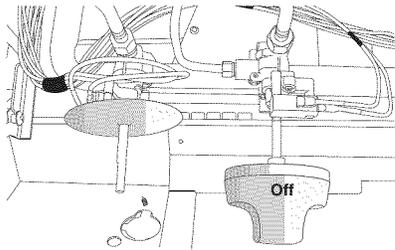
10. Turn the control knob to LO and light the burner using a butane extension lighter.
