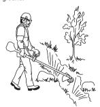
5 Keep a good balance and a firm foothold. Do not overreach. Keep proper footing and balance at all times. 6 Always hold the machine with both hands. Hold the machine on the right side of your body. Keep all parts of your body away from the hot surfaces. Keep all parts of your body away from the rotating cutting attachment.
