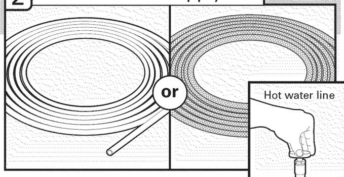
Measure overall length of copper tubing or flexible braided water supply line. Attach to the hot water line using a connection configuration that is in compliance with local codes and ordinances. The water line to the dishwasher should have a manual shutoff valve.
