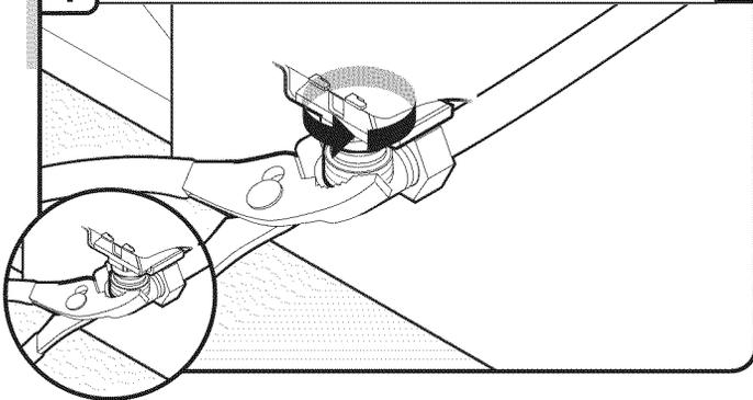
Be sure rubber washer is properly seated in fitting. Slide the  $\frac{3}{4}$ " fitting up to the valve and hand tighten to avoid cross-threading. Hand tighten until the coupling is tight. Using pliers, check the tightness of the coupling. An additional  $\frac{1}{4}$  to  $\frac{1}{2}$  turn may be required to seal the rubber gasket.
