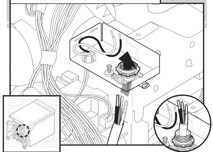
Route cord so that it does not touch dishwasher motor to lower part of dishwasher tub. Pull cord through strain relief in terminal box. Take notice when installing or removing the dishwasher in order to reduce the chance of damaging the power supply cord.
