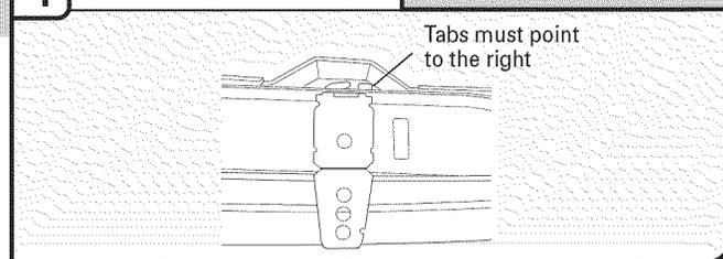
Remove the brackets from the package and place in the open slots on the left and right-hand top of the dishwasher collar as shown.
