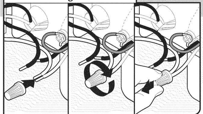
**NOTE:** Twist on UL Listed or CSA Approved wire connector. Gently tug on wires to be sure both are secured.
