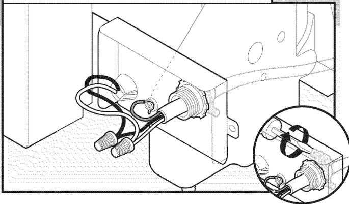
Tighten strain relief screws to secure cable.
