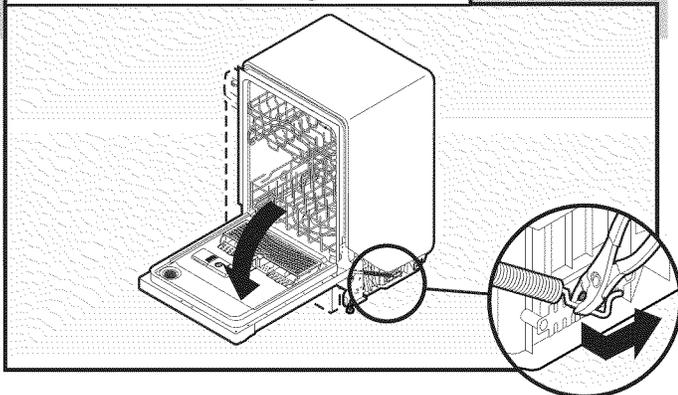
When door is unlatched, if door opens by itself, move the tensioner to a higher-numbered hole and replace the screw. Reattach door spring to rear leg.
