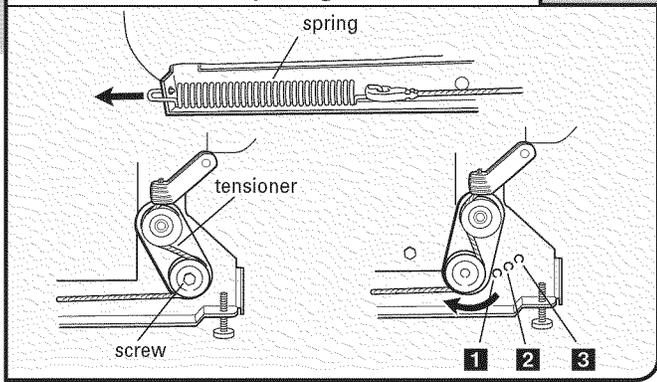
To adjust the door spring tension, unhook the spring from the rear leg of dishwasher. Using a  $\frac{5}{16}$ " nut driver or hex socket, remove the screw from the tensioner.
