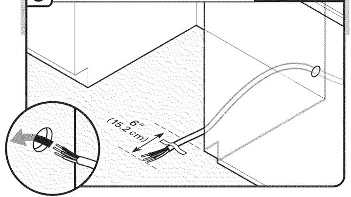
Route cable from power supply through cabinet hole (cable must extend to the right front side of cabinet opening). Tape cable to the floor in area shown. This will keep cable from moving when dishwasher is moved into cabinet opening.
