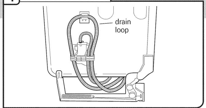
To help minimize vibration, route drain hose to avoid contact with motor, door springs, water line, cabinet, flooring or the edge of the hole where it passes through the cabinet.
