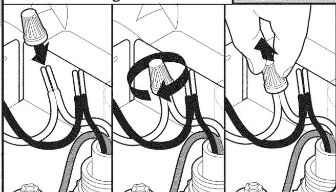
**NOTE:** Twist on wire connector. Gently tug on wires to be sure both are secured.
