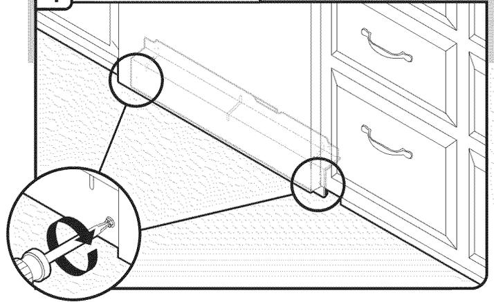
Tighten access panel screws.
