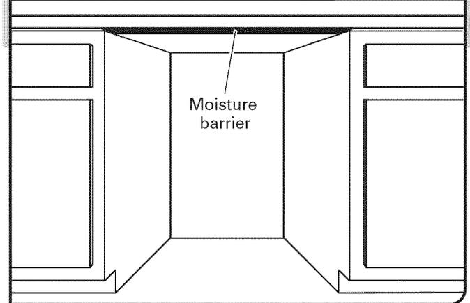
1. Make sure the area under the cabinet is clean and dry for installation of the moisture barrier.
