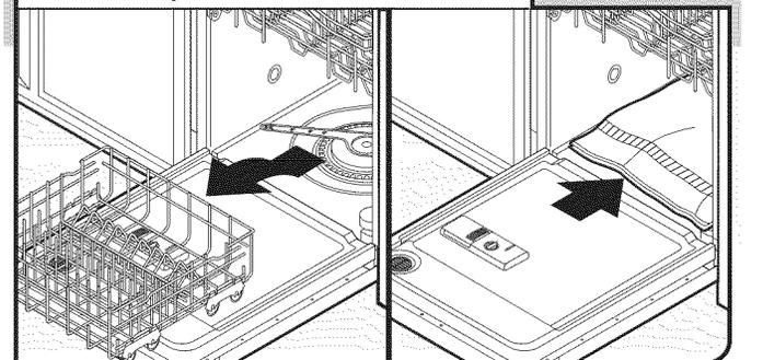
Open dishwasher door, remove lower dish rack, and place towel over pump assembly and lower spray arm of dishwasher. This will prohibit screws from falling into pump area when securing dishwasher to countertop.
