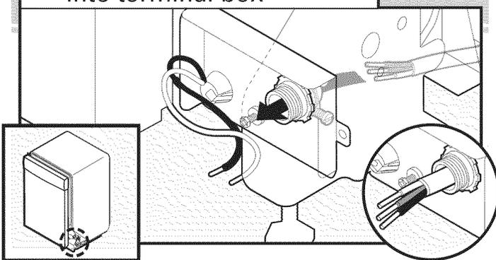
Route cable so that it does not touch dishwasher motor or lower part of dishwasher tub. Pull cable through UL Listed or CSA Approved strain relief in terminal box. Strain relief is not supplied with the dishwasher. Owner must purchase a 7/8" screw-in type strain relief.
