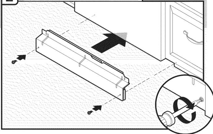
Hold the two panels together and place them against dishwasher leg. Using a Phillips or 1/4" screwdriver, reinstall the screws through the holes in the access panel and the slots in the lower panel.
