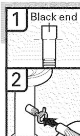
1. Connect black end of of drain hose to waste tee and cut if needed. (Do not cut ribbed section.)
