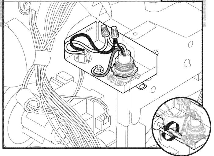
Tighten strain relief screws to secure cord.
