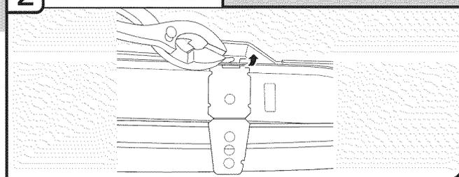
Insert the bracket into the slot on the collar. Using a pair of pliers, bend the tab down to secure the bracket in place. Repeat this step for the other side.
