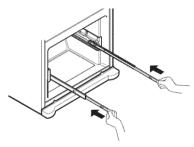
With both hands, hold each rail and push it in to allow both rails to slide in simultaneously.
