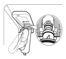
Firmly lock in the cartridge. The cover will click back into place.
