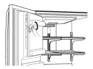
2 To remove the in-door ice bin, grip the front handle, slightly lift the lower part, and slowly pull out the bin as shown.
