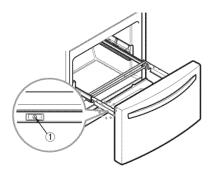
With both hands, grasp the sides of the door and pull it up to separate it from the rails.
