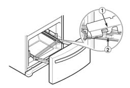
Lower door into final position and tighten the screws.
