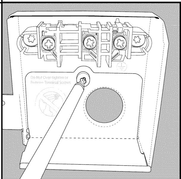
Remove strain relief plate. **Do not discard!** This will be re-installed later.
