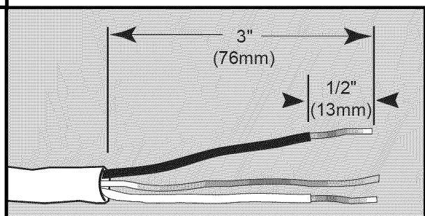
Strip outer casing of electrical wire to expose 3" (76 mm) of the inner wires. Then strip  $\frac{1}{2}$ " (13 mm) casing from each individual wire.\*
