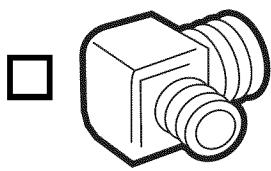
**90° elbow** with 3/8" N.P.T. male threads on one leg, and sized to fit your water supply line (copper tubing/compression fitting, or braided hose) on the other leg.
