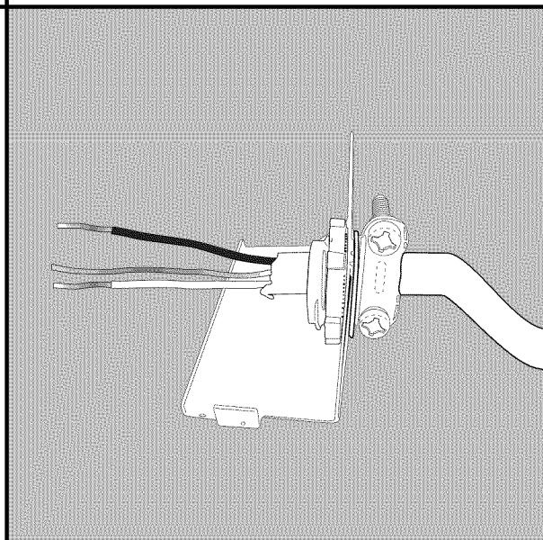
Pass wires through strain relief and plate. Tighten clamp around wires, oriented as shown. Bending the electrical cable as shown will ease installation of the strain relief plate.
