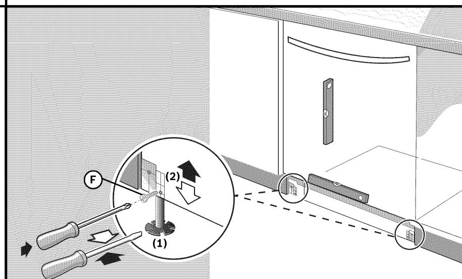
Level the dishwasher horizontally by turning feet (1) clockwise to raise or counter-clockwise to lower front of unit. Once level, (2) insert leg leveler locking screws (part F) and tighten.
