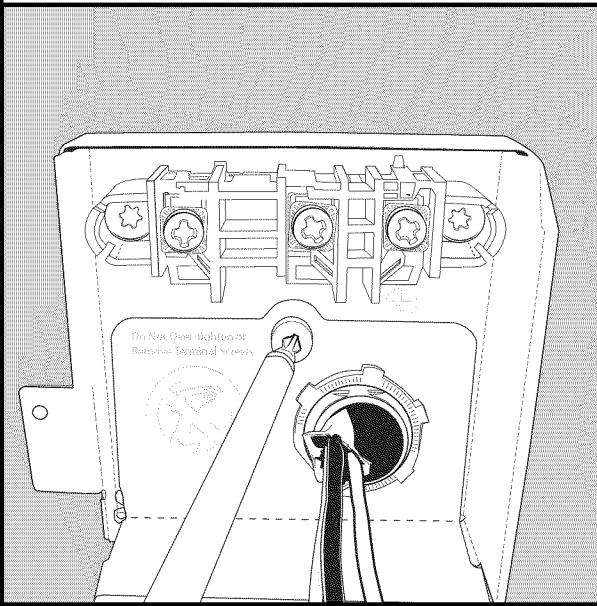
Place the assembled strain relief plate back into the junction box and re-attach the screw. Make sure the tab on the right side of the strain relief plate is outside the junction box as you slide it into place.
