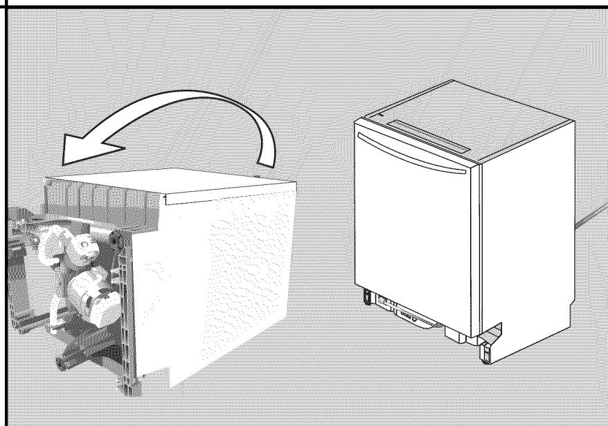
Flip unit back upright, ensuring water line is not pinched.
