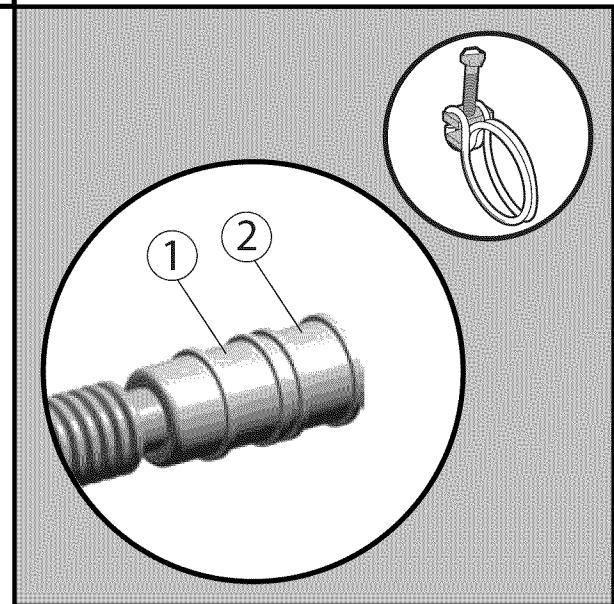
Attach drain hose to plumbing with screw clamp (position 1 for 1/2" connection or position 2 for 3/4" connection) and tighten. Do not cut drain hose.
