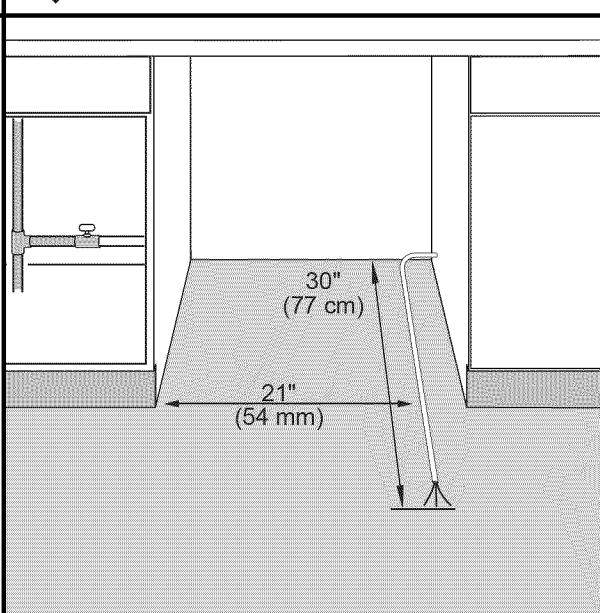
Turn power off at fuse box. Extend cable approximately 21" (54 cm) from the opening's left side. Extend the cable 30" (77 cm) from the back wall.
