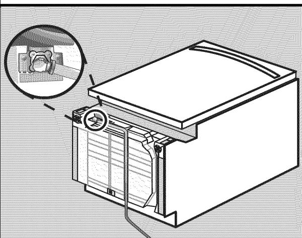
Attach hot water line to 90° elbow and route underneath machine toward hot water connection. Ensure the hose does not contact any moving parts beneath the unit.
