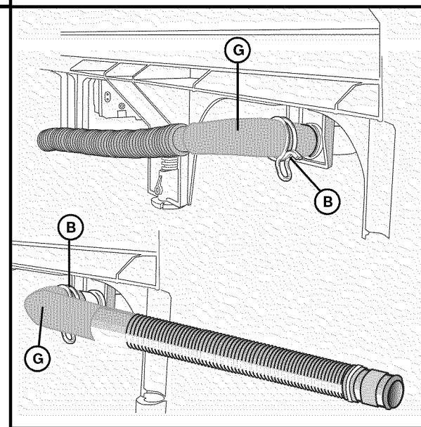
Orient hose toward direction of sink. **IMPORTANT:** Route hose toward sink PRIOR TO connection. Do not turn after attachment. Attach drain hose elbow (Part G) to back of unit using pliers to install the spring clamp (Part B).
