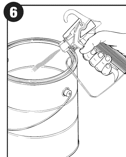
6. Continue squeezing the trigger until fluid is coming out clear. You may need to get new cleaning solution.
