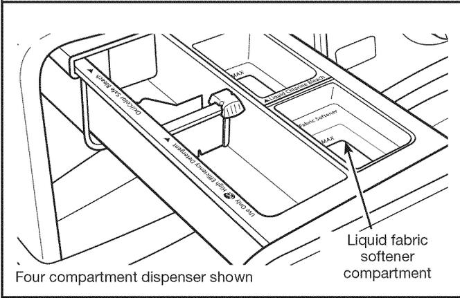
Pour a measured amount of liquid fabric softener into liquid fabric softener compartment. Always follow manufacturer's directions for correct amount of fabric softener based on your load size.
