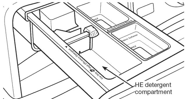
Pour a measured amount of HE detergent into detergent compartment. For powdered detergent, slide the selector to the left. For liquid detergent, slide the selector to the right.
