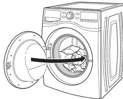
Open the washer door. Place a load of sorted clothes loosely in the washer. Items need to move freely for best cleaning and to reduce wrinkling and tangling. Close the washer door by pushing it firmly until the latch clicks.
