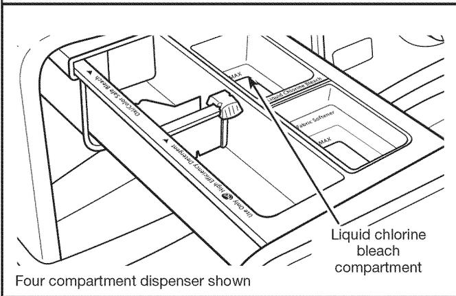
Add a measured amount of liquid chlorine bleach to the bleach compartment. Do not overfill, dilute, or use more than 2/3 cup (165 mL). Use a measuring cup with a pour spout; do not guess.
