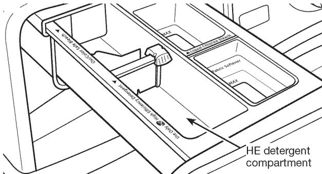
Pour a measured amount of HE detergent into detergent compartment. For powdered detergent, slide the selector to the left. For liquid detergent, slide the selector to the right.
