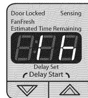
If you do not want to begin a cycle immediately, you may choose the DELAY START option. This will delay the start of the wash cycle by up to 16 hours on models with Steam, and 12 hours on non-Steam models.
