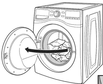
Promptly remove garments after cycle has completed to avoid odor and rusting of metal objects on garments. When unloading garments, pull back the door seal and check for small items between the tub and the basket.
