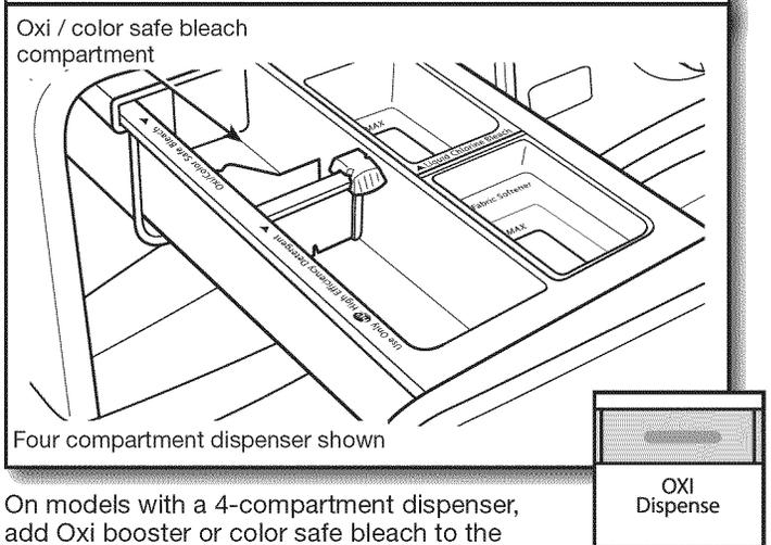
On models with a 4-compartment dispenser, add Oxi booster or color safe bleach to the Oxi compartment. Be sure to select the OXI Dispense option.
