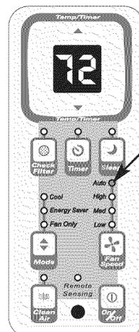
Note: Fan starts at High Speed and adjusts to a slower speed as the room temperature dictates. For example, if the room doesn't get too warm, it will stay at the slowest speed. If the room temperature rises quickly, such as a door being opened, it will automatically go to the highest speed. The fan speeds will re-adjust back to the slowest speed as the room returns to the original set temperature. Press either the fan slower or fan faster button to adjust the fan speed manually.
