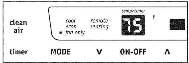
Note: Use this function only when cooling is not desired, such as for room air circulation or to exhaust stale air on some models. (Remember to open the vent during this function, but keep it closed during cooling for maximum cooling efficiency.) You can choose any fan speed you prefer. (Except "Auto Fan"). During this function, the display will show the actual room temperature, not the set temperature as in the cooling mode.
