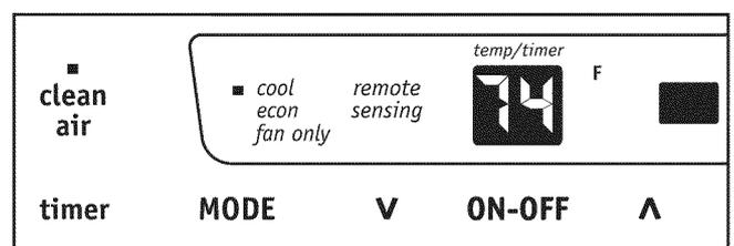
Note: When this feature is "ON", the electronic air purifier is energized to remove pollen and impurities from the air. To cancel this feature, press the Clean Air button (the LIGHT will turn off).
