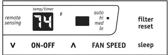
Note: Tap or hold either up ( **▲** ) or down ( **▼** ) button until the desired temperature is seen on the display. This temperature will be automatically maintained anywhere between 60 °F (16 °C) and 90 °F (32 °C) . If you want the display to read the actual room temperature. See "To Operate on Fan Only" section on Page 7.
