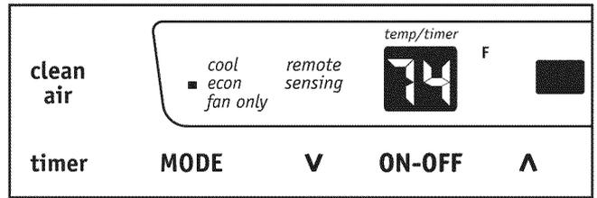
Note: In this mode, the fan will continue to run for 1 minute after the compressor shuts off. The fan then cycles on for 20 seconds at 10 minute intervals until the room temperature is above the set temperature, at which time the compressor turns back on.
