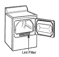
Periodically, remove the lint filter and insert the suction hose from your vacuum cleaner into the opening.
