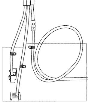
3. Remove the plastic cap from water valve inlet port.
