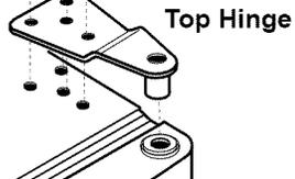
5. On 3 door (french door) models, disconnect the wiring plug located on top of the left top hinge by wedging a flat-blade screwdriver between the two sections.
