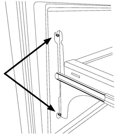
4. Lift the drawer front upward and off the screws.
