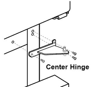
3. Place the hinge side of the refrigerator door on the center hinge pin.
