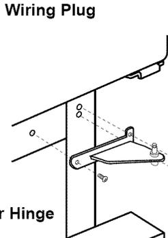
7. Remove the Phillips screws that hold the center hinge in place. Remove the hinge and retain it and all screws for later use.
