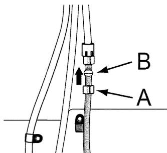
6. Slide the brass nut over the sleeve and screw it into the inlet port.
