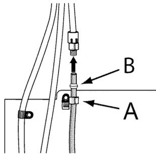
5. Place the end of the copper tubing into the water valve inlet port. Shape the tubing slightly. Do not kink the tubing so that it feeds straight into the inlet port.
