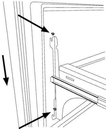
2. Tighten the four front panel screws completely. Do not over-tighten.
