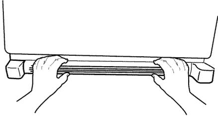
2. Using a 1/4" hex driver, turn the leveling screw on each side to raise or lower that side of the refrigerator.
