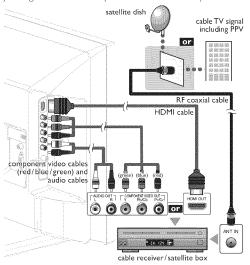
You can also connect this unit to the cable receiver or satellite box other than the HDMI or the Component Video output jacks or Composite Video output jack (IIIII p.25, 26) because they might have different output jacks.
