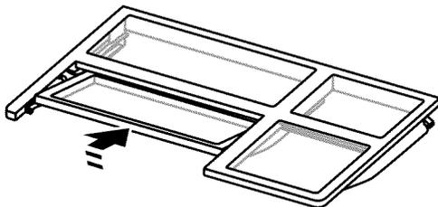
3. Replace the entire shelf by guiding it into the door liner and pushing it inward until it stops. Then, tilt the front of the shelf upward until the stopper is overcome and slide it in.
