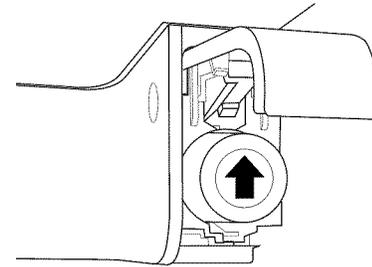
1. Locate the water filter in the top-right corner of the refrigerator compartment.
