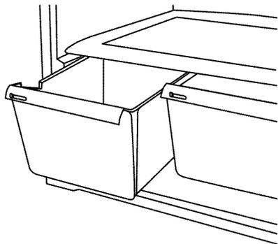
2. Lift the front of the cover to remove the cover support. Then lift the cover up and slide it out.
