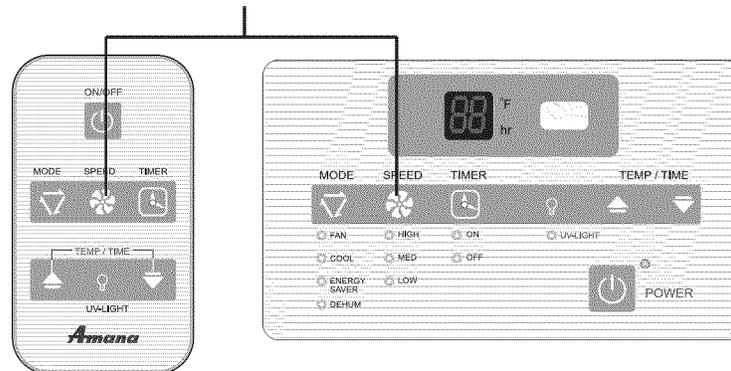
Timer on or Timer off mode is used to pre-start or shut off your unit in advance. You can program this up to 24 hours in advance. You can use the Timer in 4 functions i.e. COOL, Energy saver, Dehumid or Fan .
