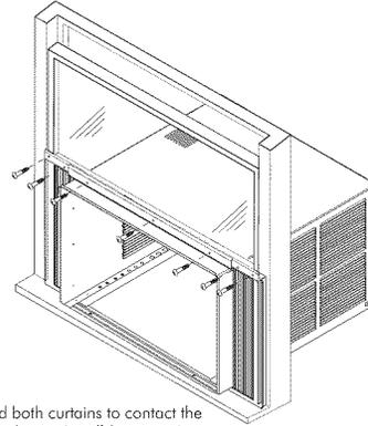
Expand both curtains to contact the window frame. Install four wood screws 31/32". Two in each upper right and left of the curtains. Install three wood screws 31/32" top mounting rail screws.
