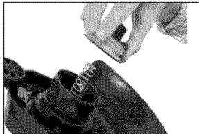
Figure 23 - Removing spool cover and spool
