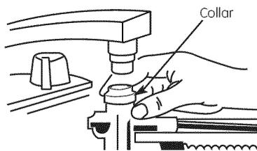
**Note:** The uniccouple's small hose carries water from the faucet to the dishwasher. The large hose carries water from the dishwasher to the sink. Orient the faucet with uniccouple attached so water from the uniccouple will run into the sink drain.
