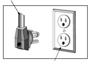
Grounded type wall receptacle (gound fault circuit not allowed)
