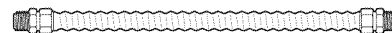
CSA-Approved Flexible Gas Line 3/8" Min. ID, 1/2" NPT Connection, 3-foot Maximum Length (Massachusetts only)
