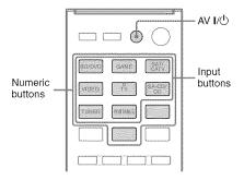
1 While holding down the input button of which you want to change the assignment, hold down AV I/1).
