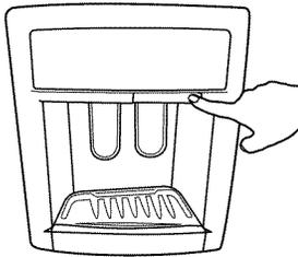
Push in on the left-hand side to rotate the faucet back into place.
