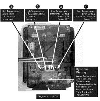
NOTE: Be careful not to select overlapping temperature settings. For example: If the HIGH TEMPERATURE LIMIT is set at 180°F with a HIGH TEMPERATURE DIFFERENTIAL set at 20°F, then the LOW TEMPERATURE LIMIT needs to be set at 160°F (180°F - 20°F = 160°F) or below.
