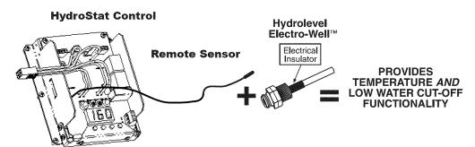
Important: The PWXL Boiler is equipped with a HydroStat Electro-Well. Do not replace the Electro-Well with a standard immersion well or the low water cut-off function will be disabled.
