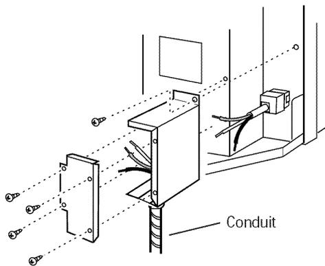
**7** If a fuse and fuseholder are to be used, the knockout at the top of the box is for mounting of a Buss Fuseholder. Be sure the fuse and fuseholder are of the same rating as the branch circuit. Leadwires at the fuse can be either soldered in place or attached using UL-listed, 1/4" female (receptacle) crimp connectors.
