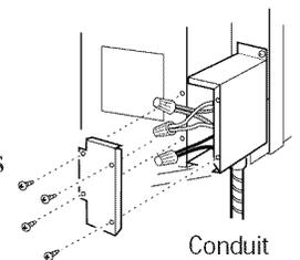
**10** Carefully tuck all wires and connections back inside the junction box. Be sure there are no loose connections or stray uninsulated wires exposed.
