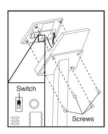
switch up or down to change the unit of measurement. Reattach the console with the four screws; be careful not to pinch any of the wires.
