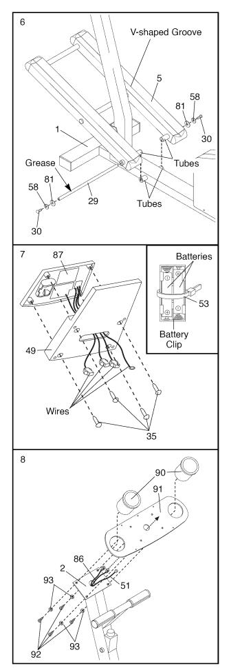
9. Connect the Extension Wire (51) to the corresponding wire on the Console (87).
