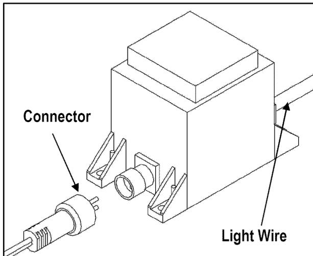
Pull the factory wire through the opening in the rear panel, plug the transformer in any household outlet.
