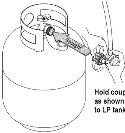
Hold coupling nut and regulator as shown for proper connection to LP tank valve.
