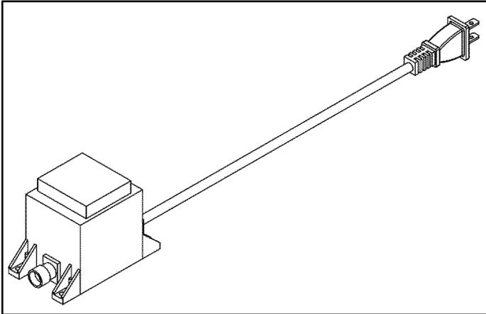
All wiring is factory connected except the easy connection you must make: connect the factory wire to the transformer with a provided screw-on plastic connector.
