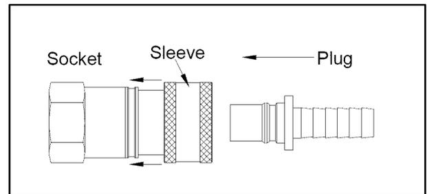
2. Insert plug and release sleeve.
