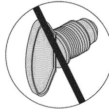
**Do not insert a POL transport plug (plastic part with external threads) into the Type 1 tank valve outlet. It will defeat the Safety Relief Valve feature.**
