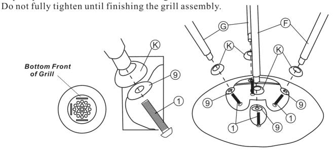
**STEP 3:** Before attaching wire shelf (J) make sure that the side with short ends is facing the front. Attach wire shelf (J) to stationary legs (F) by inserting the short ends of wire shelf (J) through holes in front legs (F), and screw 2 plastic nuts onto end tips to secure. Do not fully tighten until finishing the grill assembly.
