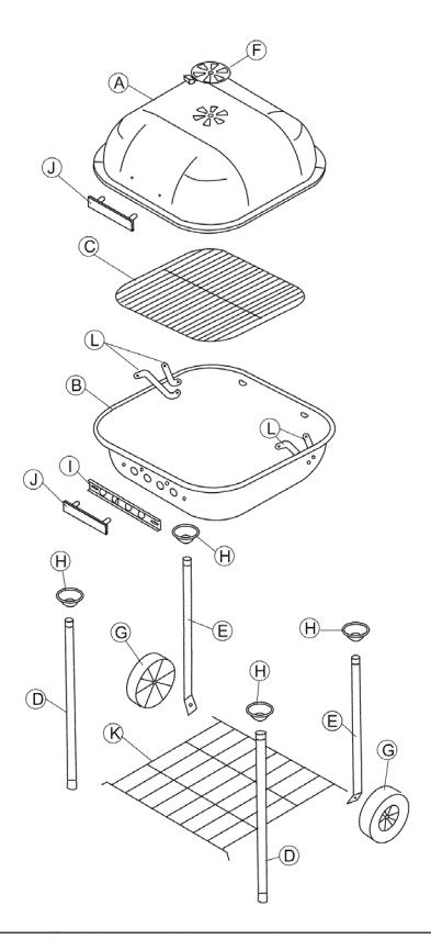
Remove all the parts from the carton and lay them out on a smooth, clean surface. Verify the presence of all parts by comparing to Hardware and Parts Lists on previous pages. Do not throw away any of the packaging until you locate all the parts.
