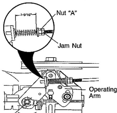
Do Not touch this nut. If further brake adjustment is necessary contact a Sears or other qualified service center.
