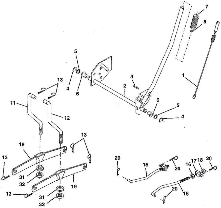
**LIFT ASSEMBLY**      **TRACTOR -- MODEL NUMBER 917.272061**
