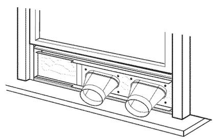
**8** Attach the bracket with a large wood screw.
