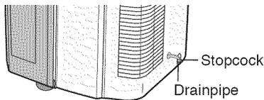
Ensure that the stopcock is securely attached the drainpipe.
