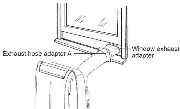
The exhaust hose should be as short as possible for operational efficiency; however, it must not be twisted or bent.
