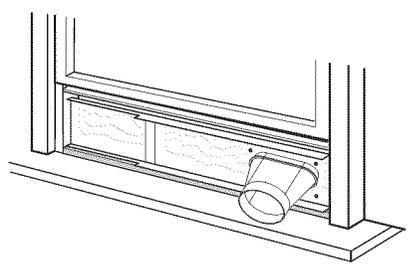
**8** Attach the bracket with a large wood screw.
