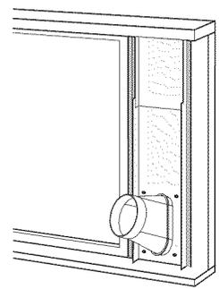
**8** Attach the bracket with a large wood screw.
