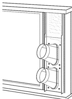
**6** Cut the foam seal B to the proper length and attach it to the window panel.
