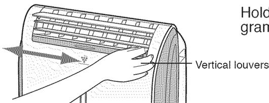
Hold the vertical louver as shown in the diagram and adjust the air flow direction.
