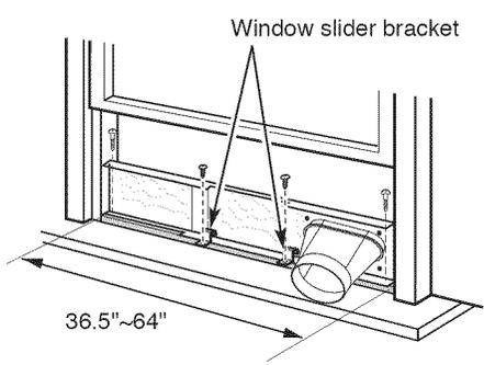
**6** Cut the foam seal B to the proper length and attach it to the window panel.
