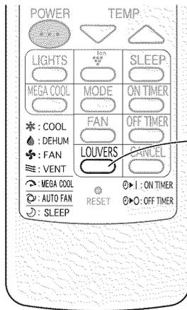
**1** Press the **LOUVERS** button on the remote control.
