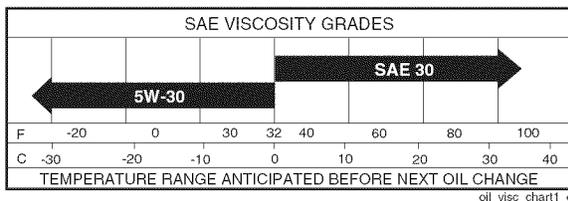
**NOTE:** Although multi-viscosity oils (5W30, 10W30 etc.) improve starting in cold weather, they will result in increased oil consumption when used above 32°F/0°C. Check your engine oil level more frequently to avoid possible engine damage from running low on oil. Change the oil after every 25 hours of operation or at least once a year if the tractor is not used for 25 hours in one year.
