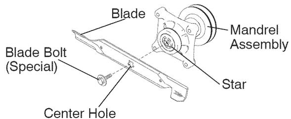
**IMPORTANT:** Special blade bolt is heat treated.
