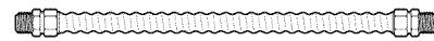
CSA-Approved Flexible Gas Line 3/8" Min. ID, 1/2" NPT Connection, 3-foot Maximum Length (Massachusetts Only)
