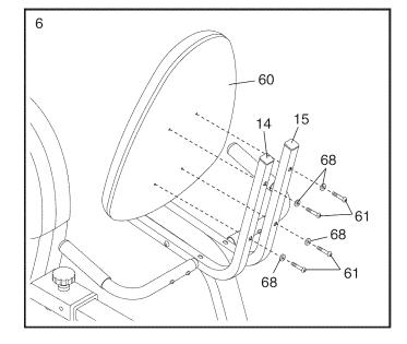
Attach the Seat (12) to the Seat Brackets (14, 15) with four M6 x 35mm Button Screws (61) and four M6 Washers (68).
