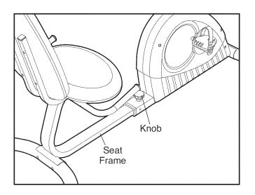
To adjust the seat frame, first loosen the adjustment knob on the frame. Slide the seat frame forward or backward to the desired position. Then, retighten the adjustment knob.
