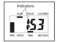
second indicator will show which information is currently displayed. Note: If you have selected a different mode, press the Display button repeatedly to reselect the Scan mode.
